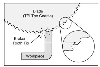
Figure 17. TPI too coarse for workpiece.
